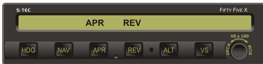
Fig. 3-31. AP Display, REV APR Mode Engaged, Track LOC Front Course Outbound
