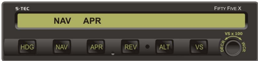
Fig. 3-35. AP Display, NAV APR Mode Engaged, Track VOR Front Course Inbound
